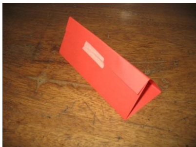
Figure 2: A4 card folded and taped to form the support for the ruler.
